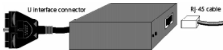
Connecting the U interface connector and RJ-45 cable
